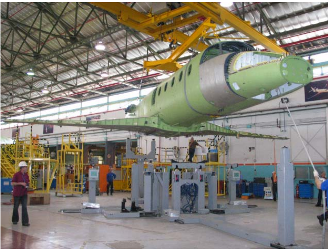
Figure 3. G150 Join Cell overall front photograph
