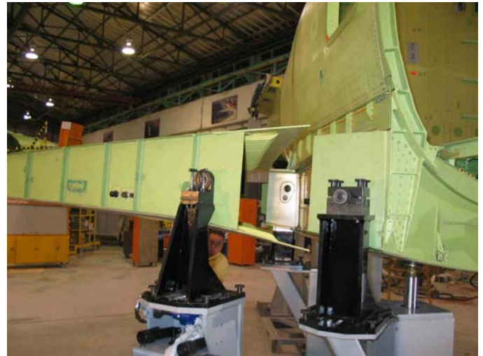
Figure 32. Wing front spar and CTS interface photo
