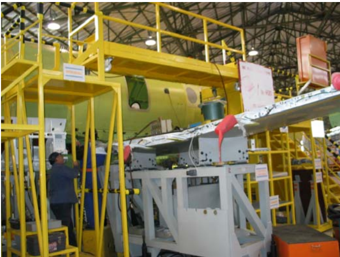
Figure 44. G200 Join Cell, right wing support and scaffolding.
