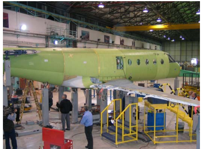
Figure 46. G150 Join Cell, right wing support and scaffolding.
