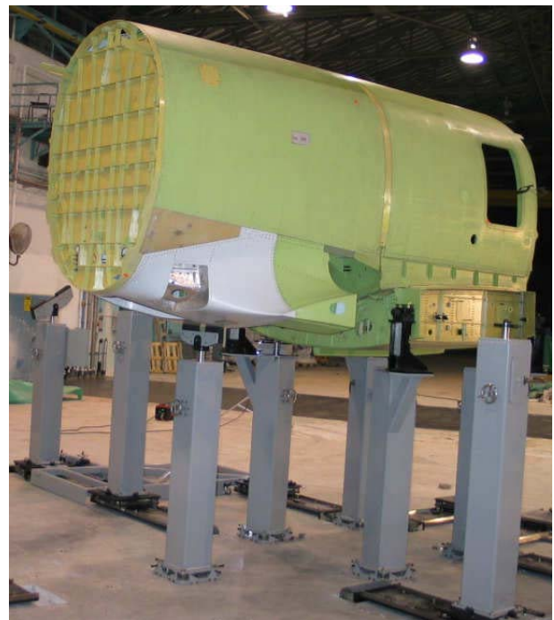
Figure 5. Center Fuselage Section loaded in join cell, side view
