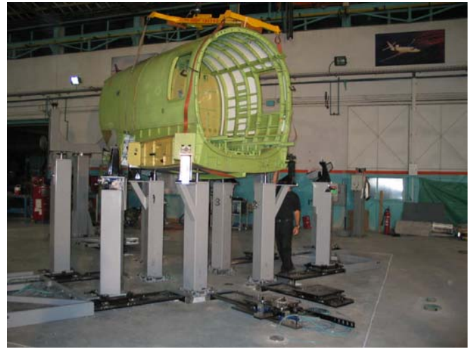
Figure 4. Center Fuselage Section loading into join cell, front view
