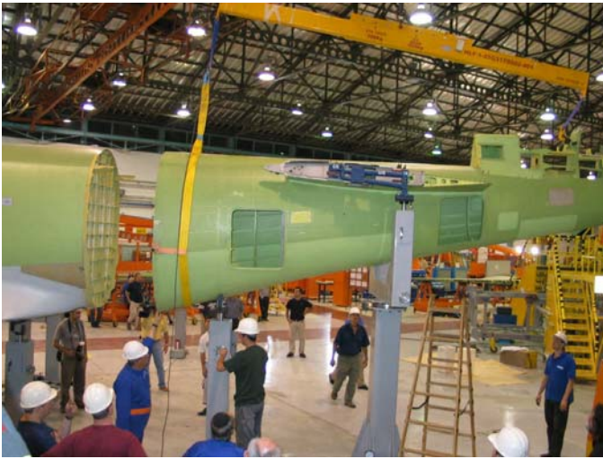
Figure 47. Aft Fuselage Loaded 0.85 m from CTS
