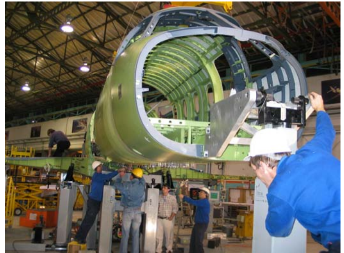
Figure 45. G150 Join Cell, front view
