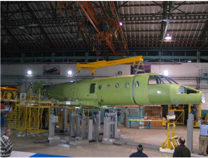
Figure 2. G150 Join Cell overall side photograph
