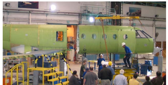
Figure 12. Fore fuselage loaded 0.85m from CTS
